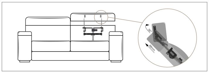
Benefit: VERTICAL spin easy motorized is an evolution of the VERTICAL motorized headrest. Easy to use, compact and the avant-garde technology makes this product unique. Equipped with a translating movement (88mm) that increases
