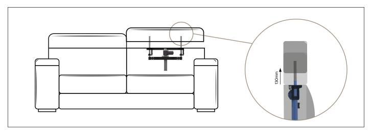
**Benefit:** The **Vertical fly** motorized headrest is a motorized translating mechanism, that allows to adjust the height of the headrest at will. New product of the VERTICAL family, the fly version is lighter and more compact, with an increased translation movement compared to the other products (130mm). Versatile and comfortable, it can be customized with a selection of TEXAS sofa joints, combining the translation with the rotation, enriching the quality of the product.
