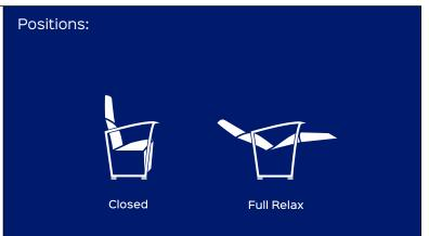
Benefit: This mechanism has been specifically designed to guarantee the maximum comfort. An actuator regulates the different positions: closed and full relax. The actuator extends the footrest and performs a slight tilting action of seat and backrest; then, it reclines the backrest reaching the maximum comfort position. TAURUS classic telescopic M1 as been designed to create padded CLOSED BASE (low foot).
