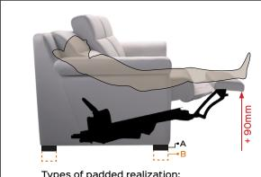
Types of padded realization: A. Low Foot (Padded closed base) B. High Foot (up to 150mm)
