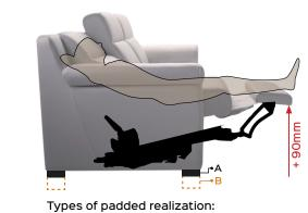
A. Low Foot (Padded closed base) B. High Foot (up to 150mm)
