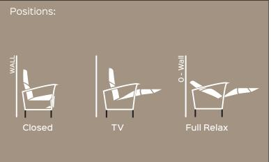
Benefit: With SUITE compact ext. footrest the relaxation experience is even more complete. op version of the SPAZIO family, the mechanics is innovative because the footboard is able to lift even more: ninety millimeters compared to previous versions. In addition, thanks to the presence of a revised flap, the footboard area is longer (+50mm). This peculiarity means that in closing, it does not remain parallel to the floor but to
