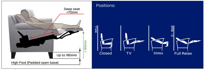
Benefit: The mechanism SUITE D.S.C. two motors is ideal for upholstered with a more compact seat. The reduced thickness allows to choose among a wide range of designs of the finished product. The presence of two motors allows to release the operation of footboard and seat (which move in a synchronized manner) from that of the backrest (which is driven by a dedicated engine). By operating the actuators you can choose, therefore, whether to recline the backrest
