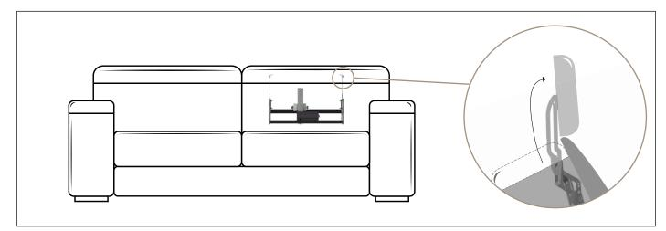
**Benefit:** The STILE extended plus motorized headrest is the flagship product of the STILE family. It's one of the most revolutionary and functional products with 102° rotation, 232mm lift and 83mm translation. This headrest guarantees a hight comfort level in all its different positions, from the Tv
