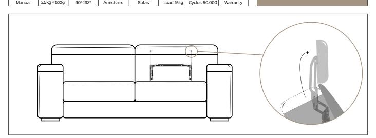
**Benefit:** The STILE extended plus manual headrest is the flagship product of the STILE family. It's one of the most revolutionary and functional products with 102° rotation, 232mm lift and 83mm translation. This headrest
