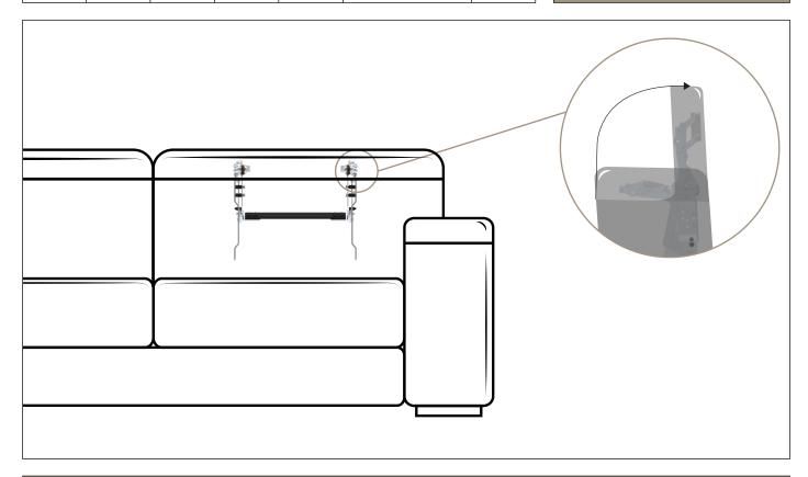
**Benefit:** The manual headrest inside the couch, the extremely compact structure has the following features: rotation 76°, raised 135mm, travel 91m. The high quality of the materials and electrical components used make
