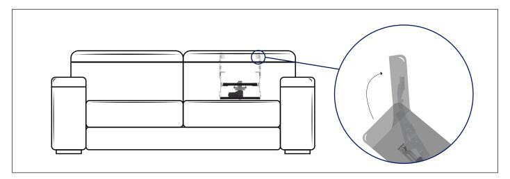
Benefit: This motorized headrest is fully upholstered inside the sofa. The very slim structure has the following features: 57° rotation, 54mm shift and 105mm translation. High quality materials and electric kit make this mechanism
