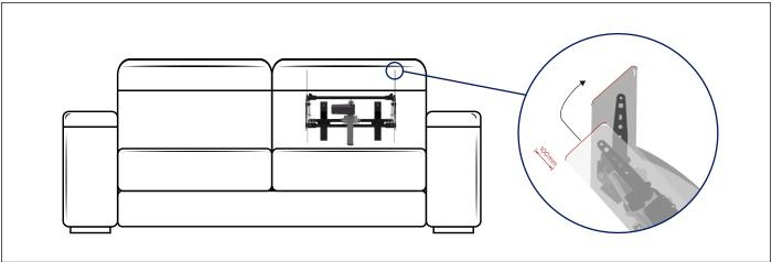
Benefit: The SPIN UP reinforced motorized electric headrest/backrest responds to the need to use it inside seats greater than 630 mm. The reinforced version has the same characteristics as the "standard" version: the levers perform a translation of 100mm and a rotation with an angle of 43° and this version is also equipped with a safe
