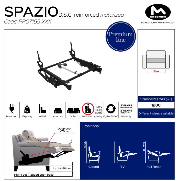
Benefit: SPAZIO D.S.C. motorized is the compact version (of 40 mm) of the homonymous SPAZIO D.S. In fact, as in the version D.S., the D.S.C. (Deep Seat Compact) is characterized by a deeper seat (+70mm) that in combination with the flap, allows manufacturers of padding to be able to use a single mattress keeping the same width between the seat and footboard. This mechanism, designed for the most spacious
