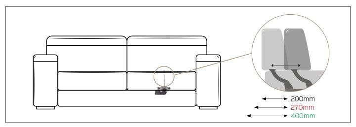
Benefit: Motorized backrest support caraterized by high efficiency and quality of the materials and of the electronic components. Its linear movement allows for the backrest to move, differnt configurations 200mm, 270mm e 400mm forward. Different relax position for the most demanding consumer. The Sollievo motorized mechanism is suitable for innovative and contemporary designs.
