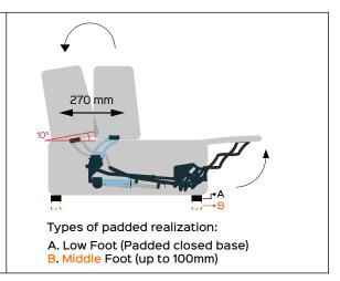
Benefit: SCORPION recliner motorized is the evolution of the homonymous mechanism SCORPION motorized. The peculiarity of this mechanism is to combine the characteristics of a mechanical with those of a backrest. The extreme simplicity of use and the elegance of the movement make its use unique. The synchronized motorized movement between the mechanics and the backrest, once actuated, increases the seat depth of 270mm as in the "manual" version,
