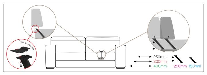
**Benefit:** SCHIENALETTO motorized is a versatile and reliable product, available in different configurations. The backrest support allows to increase the depth of the seat, depending on the user's needs. The available strokes are: 250 mm, 300 mm and 400 mm. What distinguishes this product is the presence of
