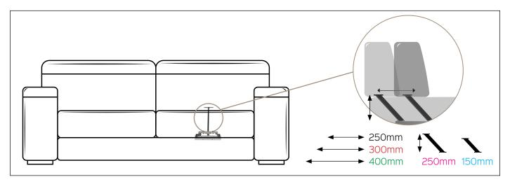
**Benefit:** SCHIENALETTO manual is a versatile and reliable product, available in different configurations. The backrest support allows to increase the depth of the seat, depending on the user's needs. The available strokes are: 250 mm, 300 mm and 400 mm. The "jerky" movement allows to reach the intermediate positions, carefully designed to guarantee the maximum comfort for the end client.
