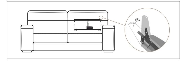
Benefit: The PUSH HEAD strong electric headrest has a strongand stable structure, it can easily fit with the design and the ergonomics of the finish product, the levers turnthrough an angle of 40° and are provided of a safetyself-returning mechanism, that stops in case of obstruction, but at the same time it allows to turn to the close phase in total security once the obstruction is removed. It's ideal to ensure a proper posture, cervical support and the best comfort.
