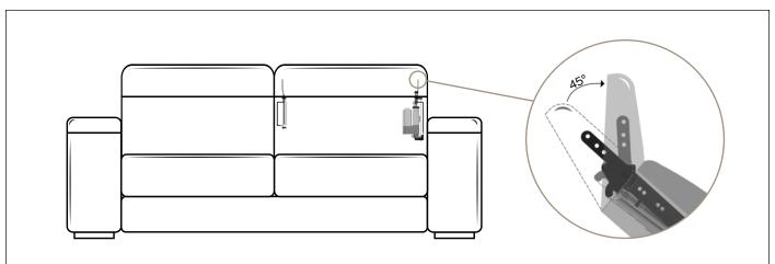
Benefit: The PUSH HEAD slim electric headrest has a strong and stable structure and compact, it can easily fit with the design and the ergonomics of the finish product, the levers turn through an angle of 45° and are provided of a safety self-
