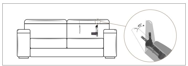
**Benefit:** The **PUSH HEAD** electric headrest has a strong and stable structure, it can easily fit with the design and the ergonomics of the finish product, the levers turn through an angle of 45° and are provided of a safety self-returning mechanism, that stops in case of obstruction,
