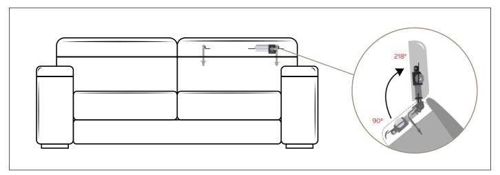
Benefit: POWER JOINT 90°-218° motorized combines the compactness of a manual ratchet with the motorized functionality, allowing it to be adjusted in any position. It also has the same size as the
