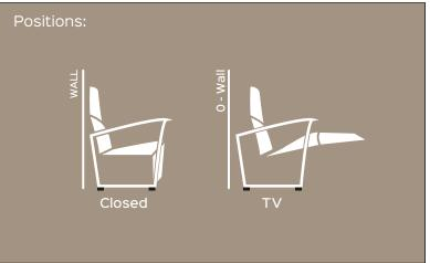
**Benefit:** ONDA slim mechanism is simple and basic. The seat and the backrest are fixed. Activating the actuator, the footrest can be moved to different positions, giving the legs comfortable postures. Various finishings are avaiable on customer's request
