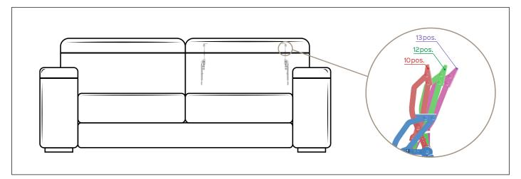
Benefit: The manual NEW CRIPTO headrest thanks to the sequential movement allows the end-user to find the best comfort position. The incorporated parts are in zinc finishing while the visible parts are chromed.
