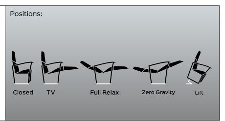
Benefit: Entry level mechanism of the Lift family designed to ensure high lifting performance and comfort, facilitating the daily life of the most needy user. Two actuators regulate the different movements in order to ensure infinite use positions, from closed to TV to full relax to lifting (lift) up to zero gravity
