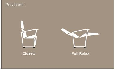
Benefit: Perfect mechanism for sofas and armchairs with clean and thin lines. With a very solid and compact basic structure, it allows the designer ample choice in the shape of the finished product. An actuator regulates the opening of the footboard and backrest in a synchronized manner. The
