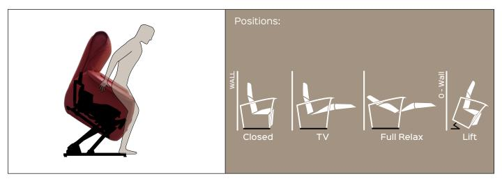
Benefit: This lift mechanism has been designed to guarantee the high lift performance and maximum comfort. An actuator regulates the different positions: closed, TV, relax and lift. The actuator extends the footrest and performs a
