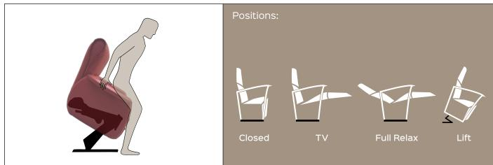
Benefit: MO-311 LIFT M2 is designed to ensure high lifting performance and comfort, facilitating the everyday life of the most needy user. Two actuators regulate the different movements in order to ensure infinite positions of use, from Closed to TV to Full relax up to the Lift. The first actuator, in addition to bringing the padded to the Lift position, extends the footboard by doing a light tilting action to the seat and
