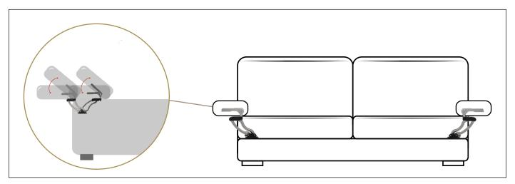
**Benefit:** MITICO evolution + sofa joint manual is a versatile product, suitable for all types of upholstery. With a simple movement, it allows to move the armrest horizontally of 275 mm increasing the vacuum of the seat. Moreover, thanks to the
