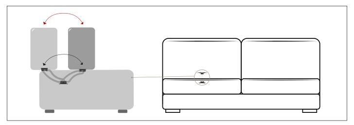
Benefit: The Mitico 260 manual mechanism can fit in chairs and sofas. it allows, with a simple movement, to shift back the backrest of 260 mm, increasing the depth of the seat.
