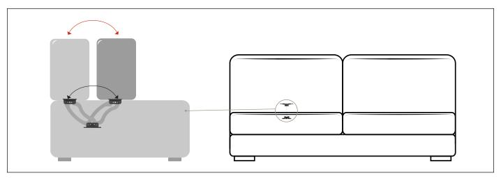
Benefit: The Mitico 287 manual mechanism can fit in chairs and sofas. it allows, with a simple movement, to shift back the backrest of 287 mm, increasing the depth of the seat. The use of high quality materials, and the simple but resistant structure, make this product easy to install and long-lasting; the visible parts are characterised by a chromed finishing.
