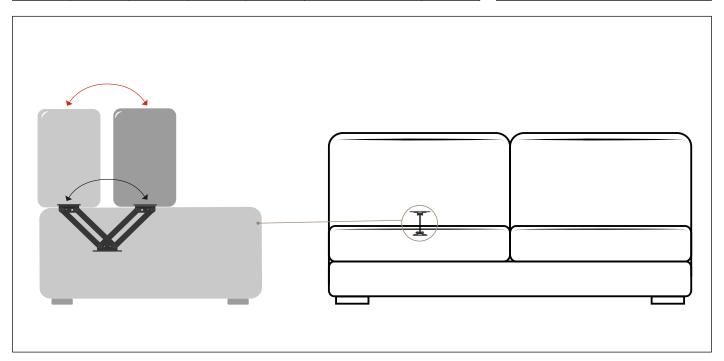
Benefit: The Mitico 260 manual mechanism can fit in chairs and sofas. it allows, with a simple movement, to shift back the backrest of 260 mm, increasing the depth of the seat. The use of high quality materials, and the simple but resistant structure, make this product easy to install and long-lasting; the visible parts are characterised by a black paint finishing.
