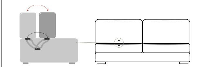
Benefit: The Mitico 260 manual mechanism can fit in chairs and sofas. it allows, with a simple movement, to shift back the backrest of 260 mm, increasing the depth of the seat. The use of high quality materials, and the simple but resistant structure, make this product easy to install and long-lasting; the visible parts are characterised by a chromed finishing.
