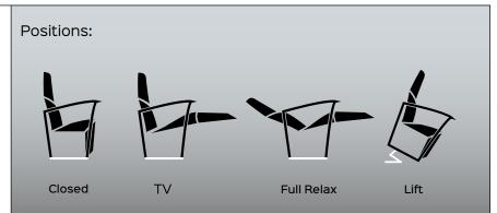
**Benefit:** The KEYMOTION mechanisms are built entirely in Italy, from the raw material, to the processing, up to the final assembly and testing. The products are carefully checked before being shipped. This mechanism is designed to ensure high lifting performance and comfort, facilitating the everyday life of the most needy user. Two motors regulate the different positions: closed, TV, full relax and lift. The first actuator, in
