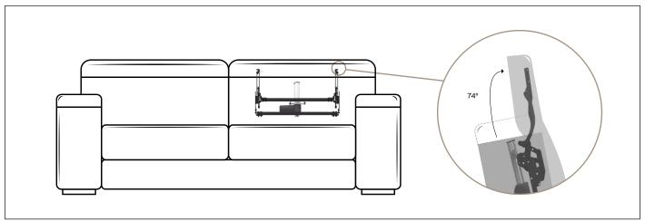
**Benefit:** Electric headrest designed for fixed seats. Highgrade and efficiency materials and electric components. Narrow shape and great versatility (74° rotation, rise
