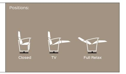
**Benefit:** A manual mechanism that is ideal for armchairs aiming for maximum comfort, with a very solid and compact basic structure it allows the designer ample choice in the shape of the finished product. Moving the product is simple, simply shift your body weight backwards on the seat to activate the mechanism and open the footrest to obtain the 'TV' position. The manual release adjusts the movement of the mechanism: from closed to full relax.
