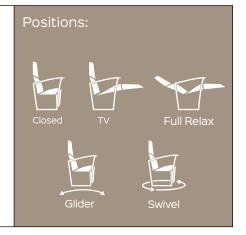
Benefit: Extremely solid and versatile mechanism, can be used on different models of armchairs, from classic to contemporary design. The mechanics is equipped with an actuator for infinite relaxation positions with the simple electric adjustment from closed, tv to Gravity 0. "Gravity 0" is the result of extensive studies that have shown that, thanks to the
