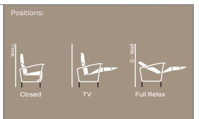
Benefit: In the double compact version, the Brio mechanics is more compact (of 40 mm than the standard version) and allows the manufacturers of upholstered furniture to design open base sofas and armchairs in a more contemporary style. The flap adds a larger extension to the pedestal while the
