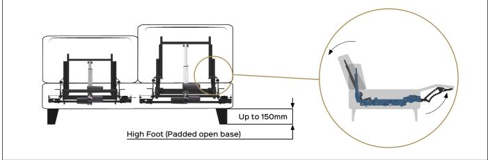
Benefit: ATTRACTION motorized combines a mechanism and a backrest. Thanks to the compact structure is perfect for OPEN BASE sofa (high feet) and chair with a contemporary design. The structure has been designed to become the frame of the furniture itself with housing for cables and control boxes.
