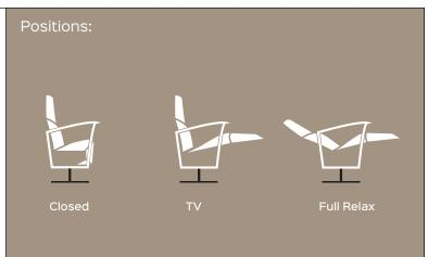
Benefit: ACTIVEX is a motorized mechanism specifically designed to ensure the best comfort. The compact and solid structure allows wide possibilities of finished products. Two actuators regulate the movement of the mechanism from closed to full relax. The combined movement technology
