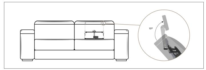
Benefit: The Action motorized electric headrest is a product of contemporary, efficient, compact design and versatile use (121°rotation, 181mm rise, 109mm shift). High efficiency of comfort in all positions, from TV to relax,
