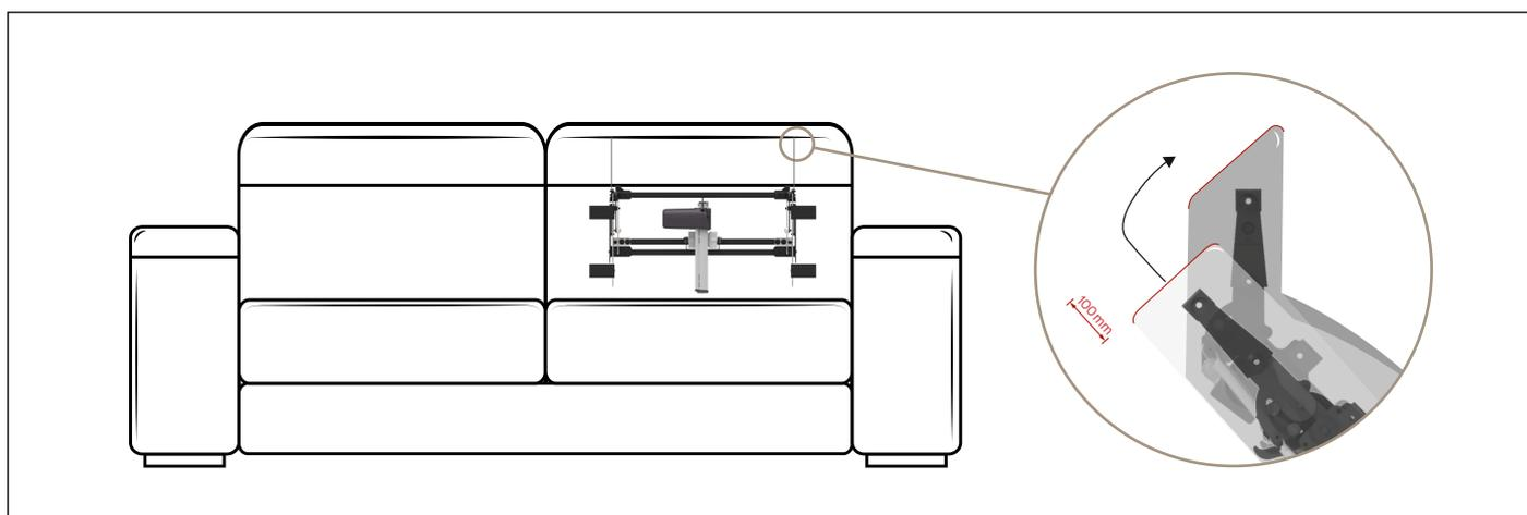
**Benefit:** The SPIN UP total back motorized electric headrest has a solid and resistant structure. The peculiarity of this product is the perfect combination between the backrest features and the headrest once, in fact, once fixed on the frame, the spin up allows a 100 mm increase of the support surface of the back in
