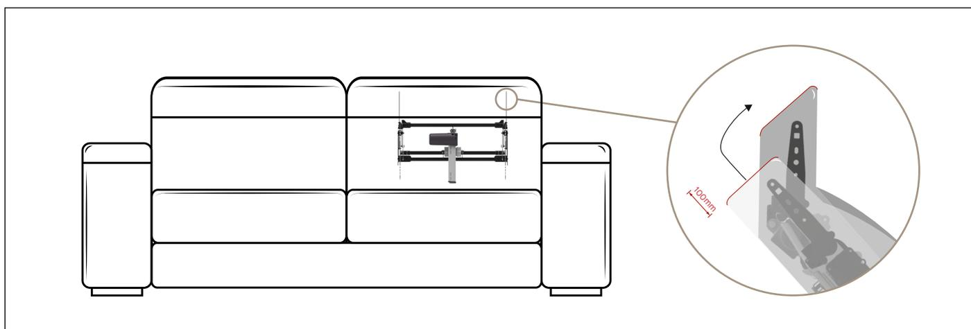
**Benefit:** The SPIN UP electric headrest/backrest has a strong and stable structure, the mechanism is designed to fit also with the aesthetics of compact sofas. The levers carry out a translation of 100 mm and turn through an angle of 43°, to create the perfect and
