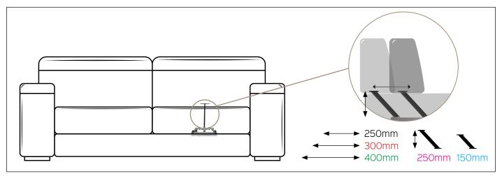
Benefit: SCHIENALETTO manual is a versatile and reliable product, available in different configurations. The backrest support allows to increase the depth of the seat, depending on the user's needs. The available
